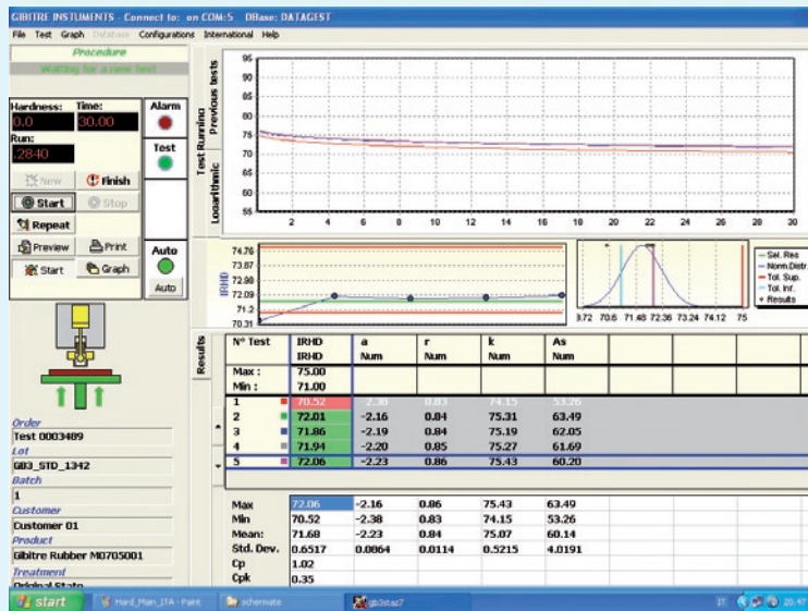
The main page of HardnessCheck software: the test curves, test results, tolerance limits. Several hardness units can be used at the same time.
